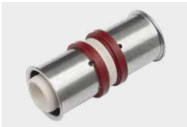
Fig. 51. KAN-therm ultraPRESS coupling for PERTAL, PEXC, PERT, bluePERT and bluePERTAL pipes 14 × 2, 16 × 2, 20 × 2, 25 × 2,5 mm.
