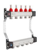
Note: The manifold works with  $G^{3/4}$ " eurocone adapters and  $G^{3/4}$ " connectors. Outlets for individual circuits have 50 mm spacing. Howmeter adjustment range 0 - 2.5 l/min.
