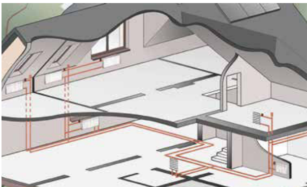
“Vertical” system in a heating installation
