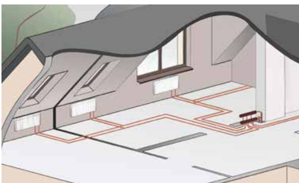
Manifold – tee system in a heating installation
