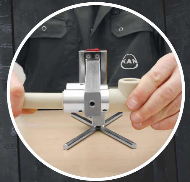
04 Heating the pipe and fitting.
