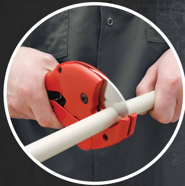
01 Cutting pipe with scissors.
