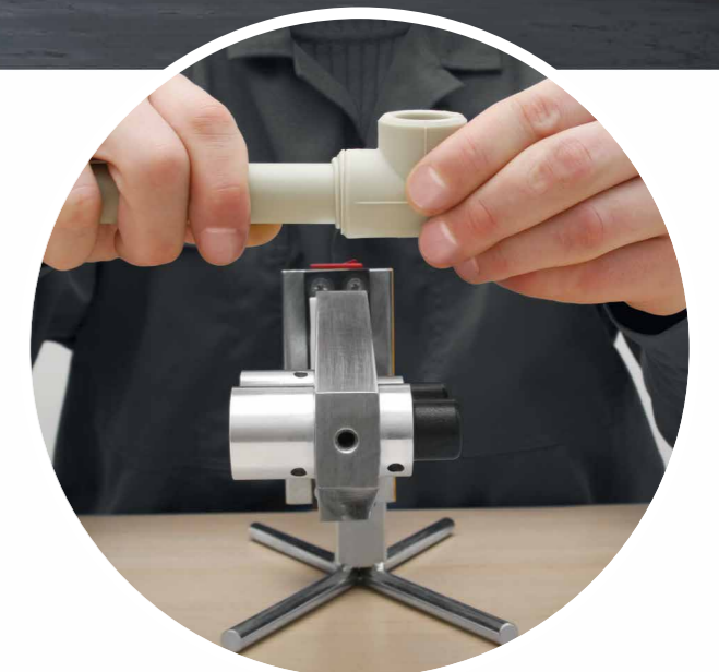
06 Fixing and cooling down the joint.
