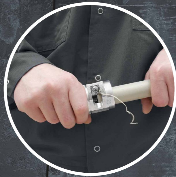
02 Removing the aluminium foil with the scraper (applicable to stabiAL PPR composite piping).
