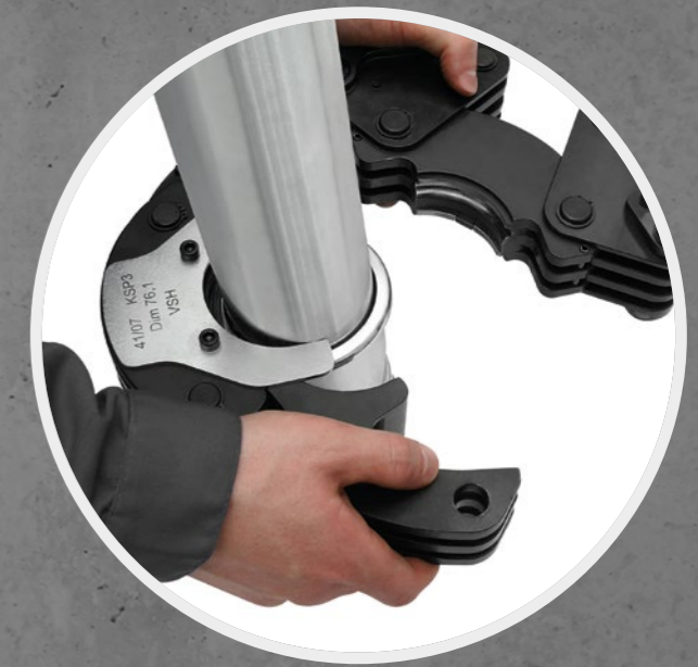
07 The jaw has a special groove into which the flange of the fitting must be fitted.
