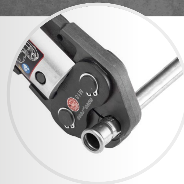
06 Preparing the jaw. The jaw, once removed from the case, must be unlocked and then unfolded.
