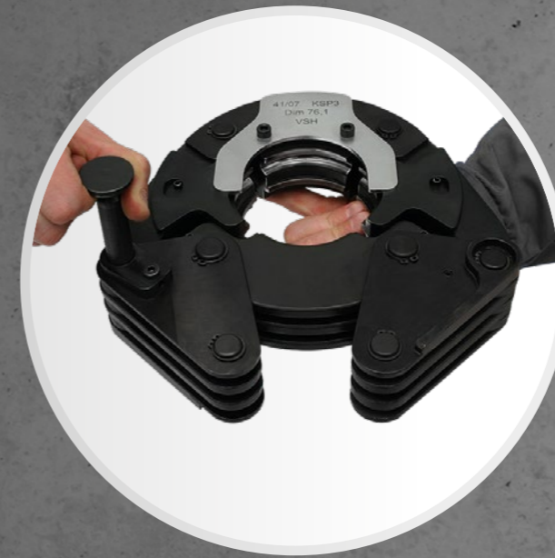
06 Preparing the jaw. The jaw, once removed from the case, must be unlocked and then unfolded.
